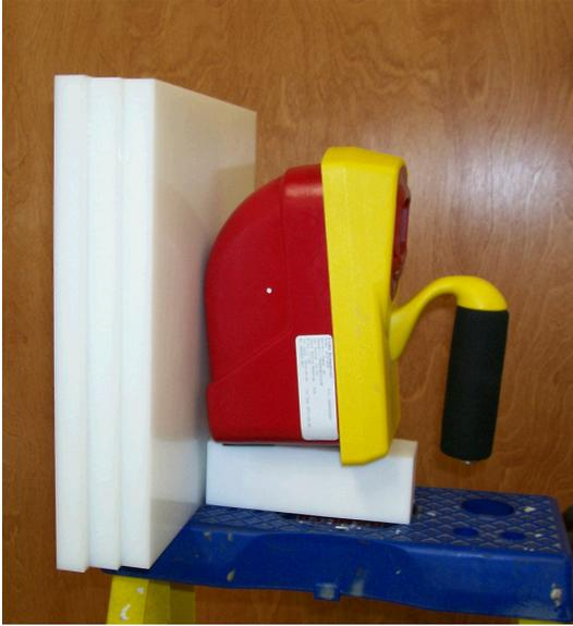
Figure 1. Photograph of a test procedure used to measure Dose Penetration.
