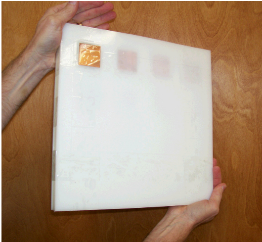
Figure 2. Photograph of a test object used to measure Imaging Penetration .
